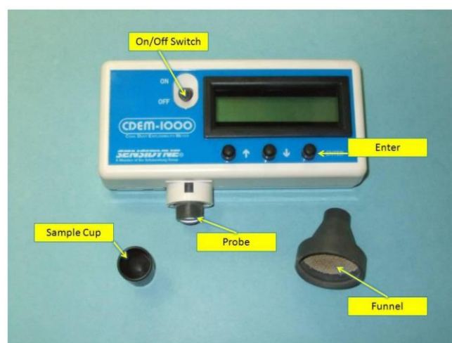
Figure 2-3 NIOSH coal dust explosibility meter (CDEM) [22]
