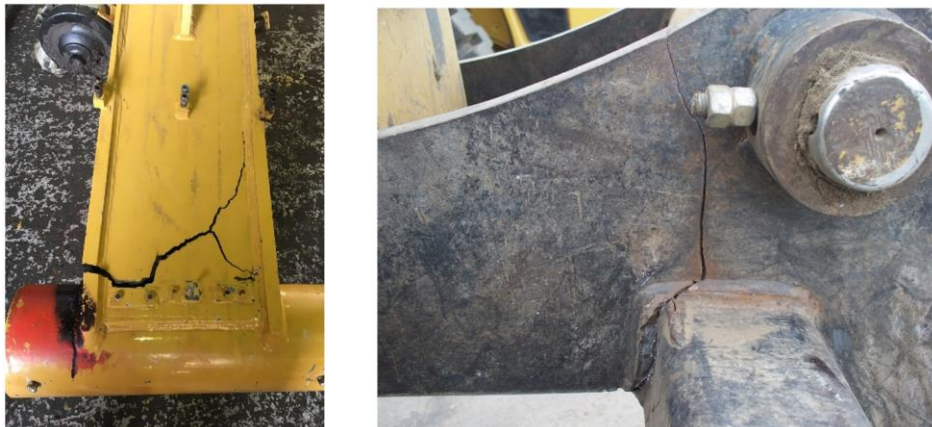
Figure 8-5 Cracks within Mining Equipment
