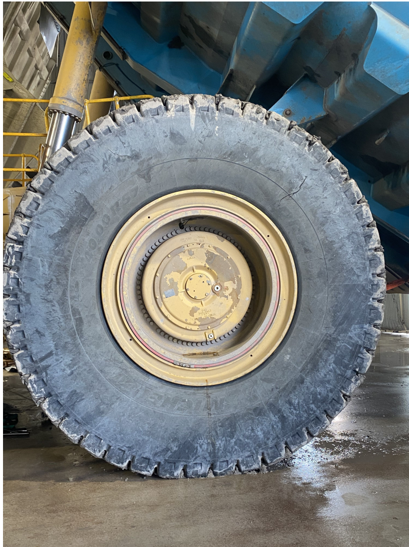
Figure A.2 – Sidewall Cut on a Liebherr Haul Truck
