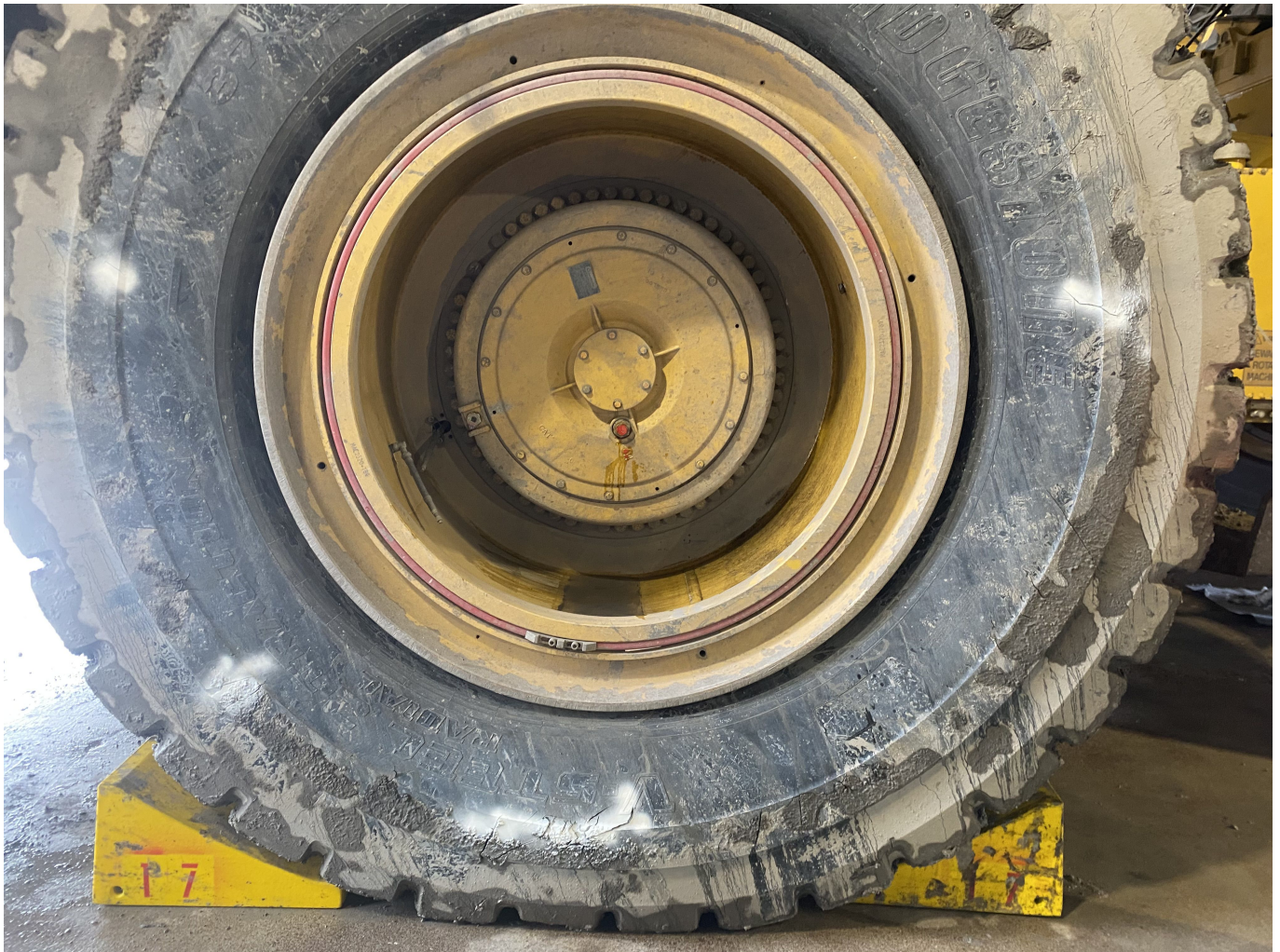
Figure 3.10 – White Markings indicating tyre issue has been recorded
