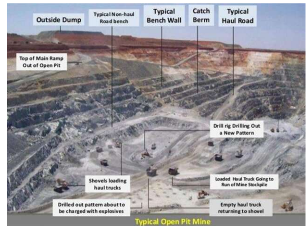
Figure 1.2 – Diagram of a surface mine [55]
