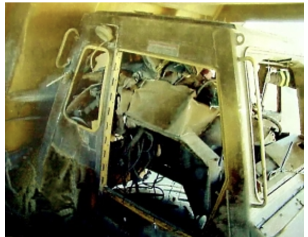
Figure 1.3 – Haultruck tyre incident that resulted in a fatal injury [86]
