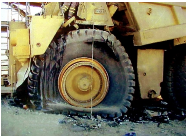
Figure 1.3 – Haultruck tyre incident that resulted in a fatal injury [86]
