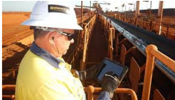
Figure D.9 – Maintenance operator carrying out a visual inspection of a conveyor belt [24]
