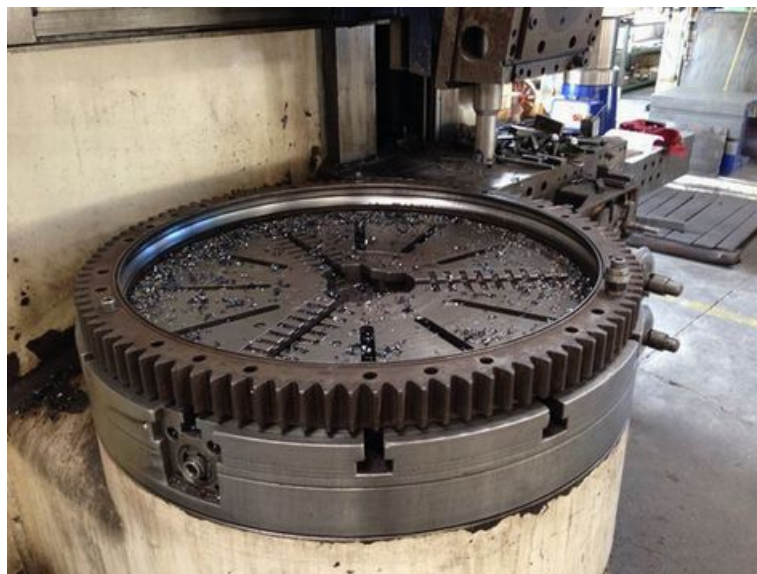
Figure D.6 – Excavator Slew Ring [13]
